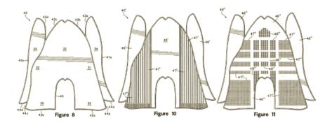
'011 patent, Figures 8, 10, 11. These figures illustrate the shape of textile element 40 before the formation of seams to create the general shape for receiving a foot. Even Adidas's expert agreed that the upper illustrated in Figure 8 "could be made on a flat knitting machine" and "then the edges that are shown in Figure 8 would be flat knitted." J.A. 1483; see also J.A. 1574 (Nike's expert
