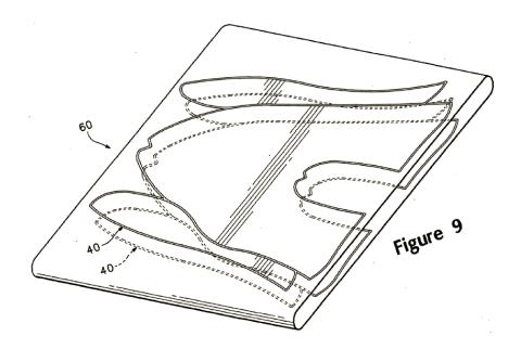
'011 patent, Figure 9. As shown in Figure 9, a circular knit upper, as distinguished from flat knit, must be removed from surrounding textile material by, for example, cutting. In addition, Nike's expert explained that the embodiment illustrated in Figure 9 is made "using a circular knitting process and requires that the textile element [40] be formed as part of a larger textile structure
