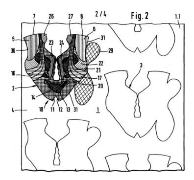
Id. at Figure 2. The process disclosed in Nishida then requires that the portion of the pattern corresponding to the shoe upper be cut from the surrounding textile web. Id. at 2:20–22. After the upper is cut out, the "cutting waste" "represents a simple, lightweight and inexpensive material." Id. Nishida therefore improves on the prior art, where the cutting waste consisted of the normal, more "expensive tubular material, multilayer material or the like." Id. at 2:24–25.
